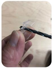
Use a 1/8 inch diameter drill bit, drill a hole through the provided mounting clip.
