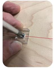
Align provided mounting clip on guide line. Use phillips head screwdriver, attach mounting clip with provided screw.
